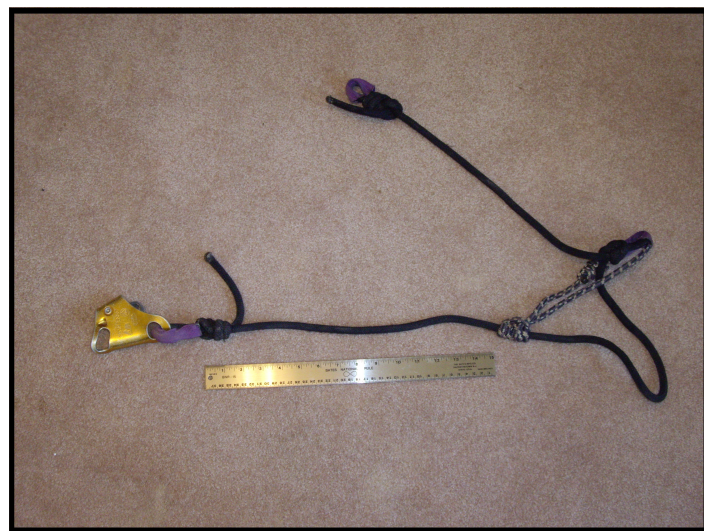
Fig. 2 - An Adjustable Ascender which has been shortened
