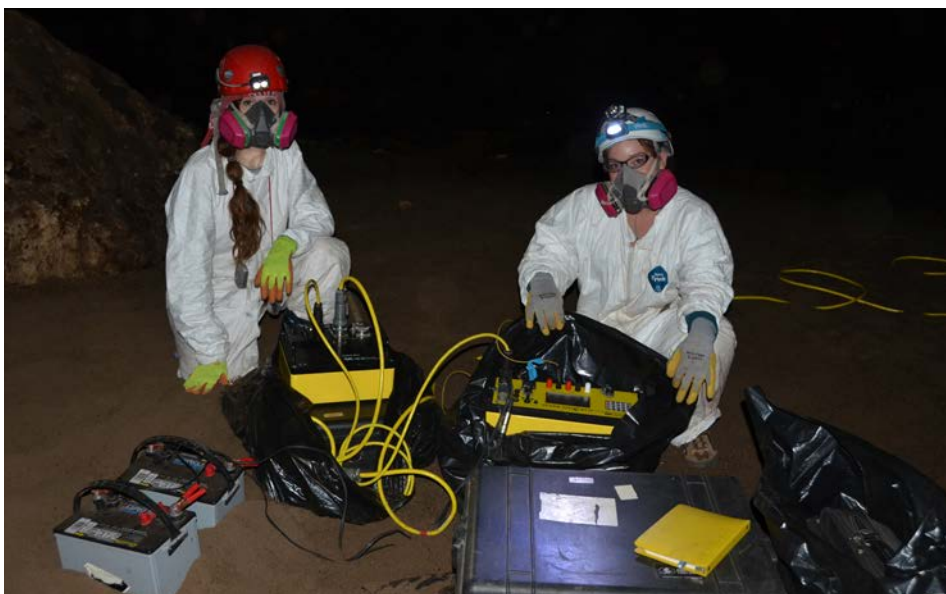
Two car batteries power the SuperSting meter (on the right in front of Jennifer Adkins - right) which connects to the cables through the switchbox (on the left in front of Jill Orr - left). A black carrying case is in the right foreground. The meter and switchbox sit inside construction-grade black plastic bags to limit contact with the guano. Photo by George Veni.
