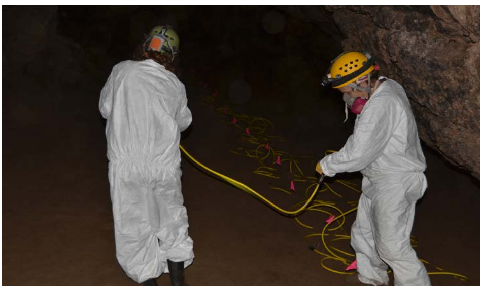
Evelynn Mitchell (left) and Linda Palit (right) carefully lay the delicate resistivity cables in the guano. Photo by Allan Cobb.
