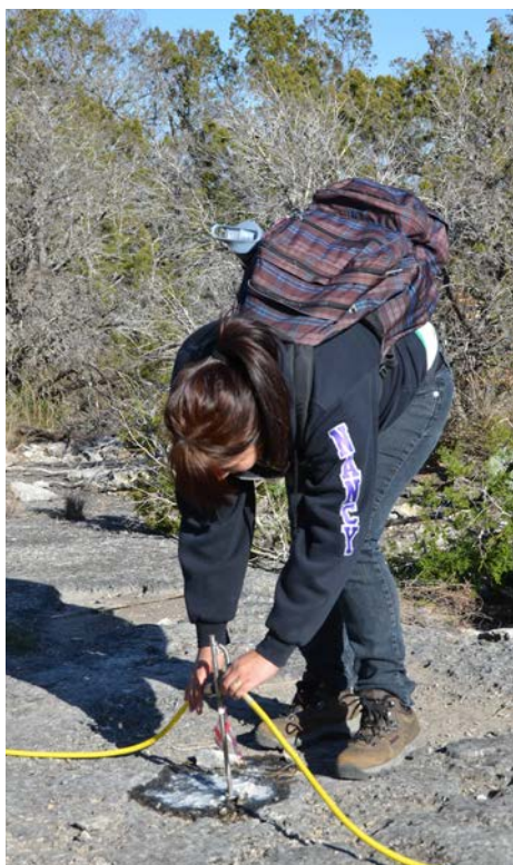
St. Mary's University student Nancy Urbano connects the resistivity cable to an electrode. Photo by George Veni.
