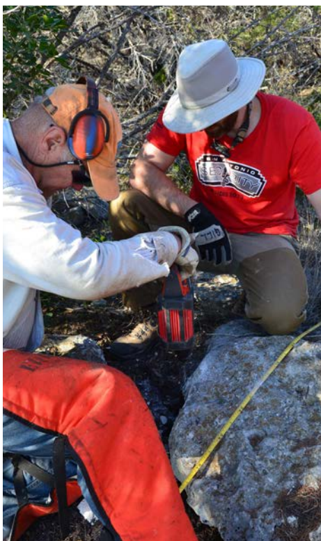
Gill Ediger and David Ochel drill into the bedrock to set an electrode. Photo by George Veni.
