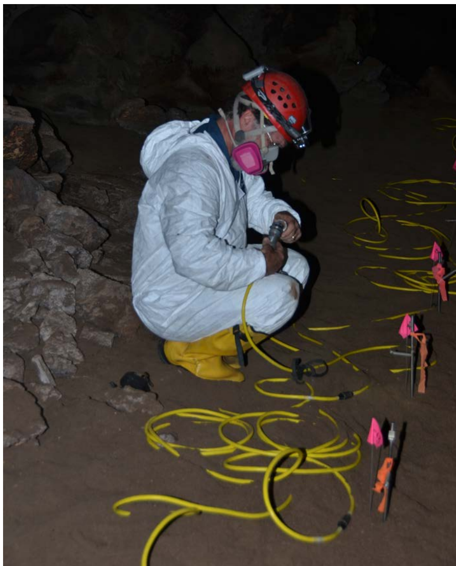
LEFT: George Veni connects two resistivity cables in Bracken Cave. Photo by Allan Cobb.
