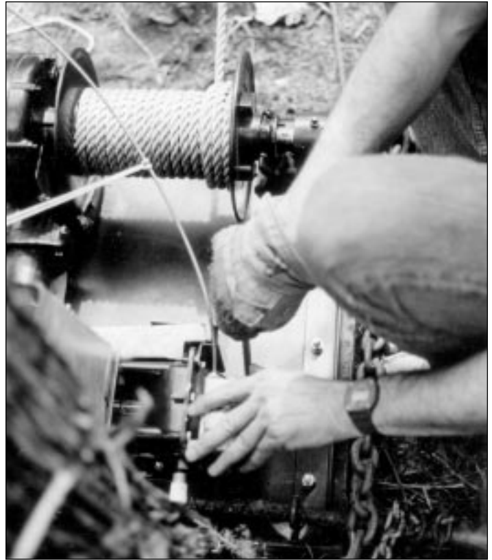
May 1990. First use of winch operated by Rick Corbell. Left hand on throttle, right hand (gloved) on shift lever. Winch double chained to tree. Buckets on end of line hauled up from 60 ft depth. Bindseil's Well near Bracken.
